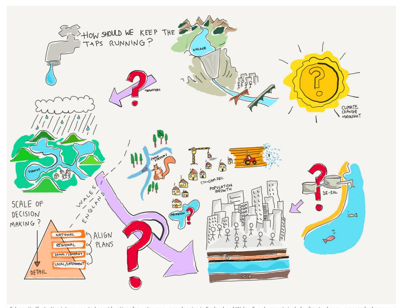
Schematic illustrating interconnected considerations for water resources planning in England and Wales. Supply aspects include climate change, proposed schemes such as desalination and the Abingdon reservoir. Supply-network related aspects include the proposed Severn-Thames transfer. Environmental aspects include the chalk streams. Demand related aspects include population growth in the Ox-Cam Arc and irrigation demands in the agriculturally productive regions in East Anglia.
